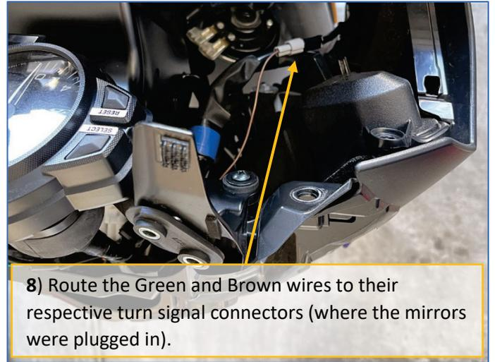
8) Route the Green and Brown wires to their respective turn signal connectors (where the mirrors were plugged in).
