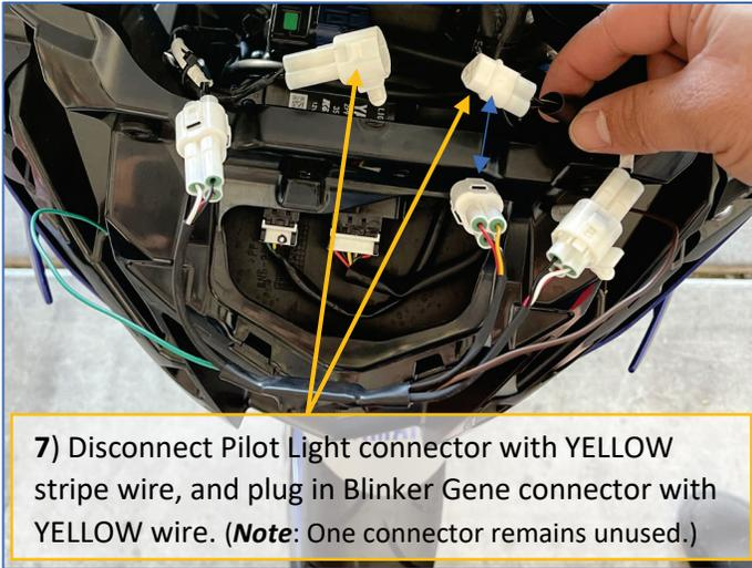
7) Disconnect Pilot Light connector with YELLOW stripe wire, and plug in Blinker Genie connector with YELLOW wire. (**Note:** One connector remains unused.)
